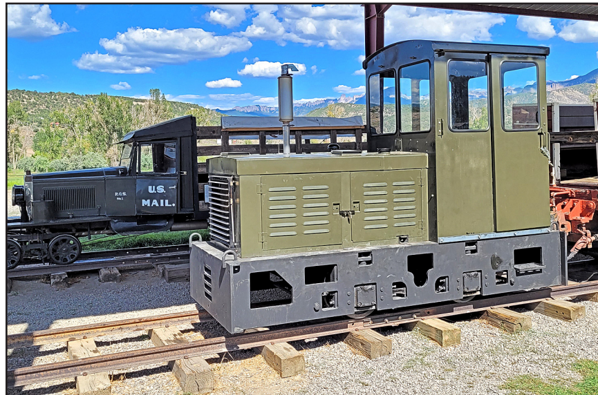
This 5-ton 1968 Plymouth (gas / hydraulic) locomotive arrived at the Ridgway RR museum in early August. It will be used for switching and pulling rider cars until they receive their replica of RGS steam engine #36. That 4-4-0 is getting closer to completion, but no delivery date is known yet. – Photo © 2022 Dave Schaaf.
